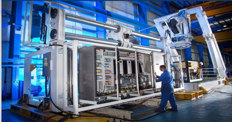
MJR Delivers Low Harmonic Deck Mounted Power, Drive, Automation & motors Solution for 12te AHC Winch with Operating Depth of 6000m
