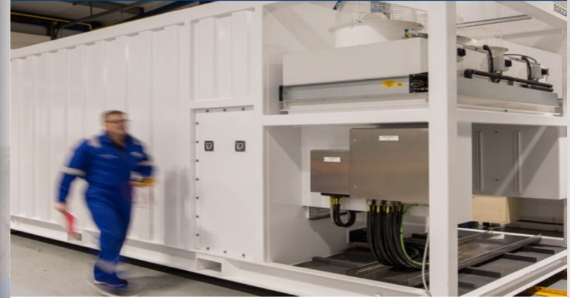
DNV2.7-1 Offshore Power Container Complete with AFE Drive Switchboard; Air-con; 3.3kV Step-up Transformers & Motors Protection Relays
