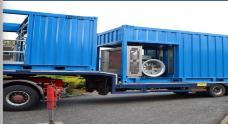
DNV2.7-1 Offshore Drive & Control Containers Complete with Drive Switchboards; MCCs; Active Harmonic Filters; Control Desks & Vessel Interface Comms.
