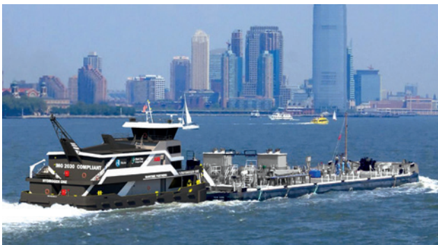
Due to be launched late 2023/early 2024, this Elliot Bay-designed tug will be hydrogen powered (1-2MW), with the hydrogen generated on board from a methanol/water mix (credit: Maritime Partners)
