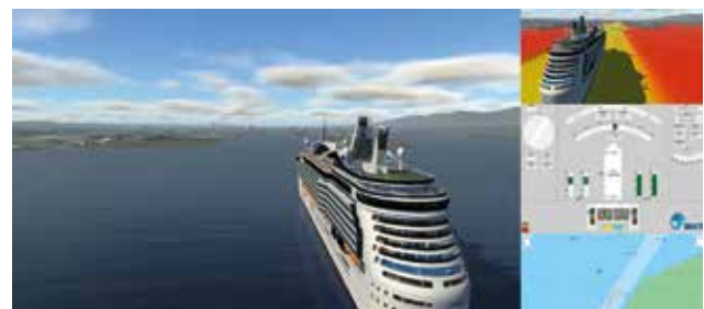
Figure 2: BMT’s REMBRANDT simulator using S-102 bathymetric data to examine port entry
